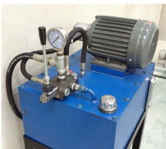
Hydraulics assembly with nonflammable hydraulic fluid
